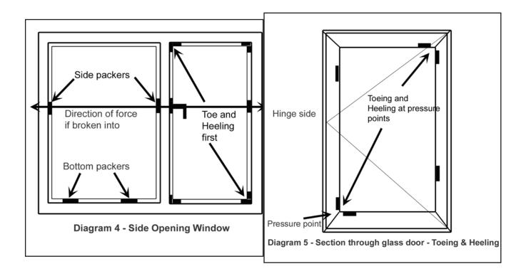
Diagram 4 illustrates a side opening window. Look at where the packers are situated. The two at the bottom of the windows (on both the left and right windows) sit the units up off the frame to prevent it sitting in water that may have seeped in.
