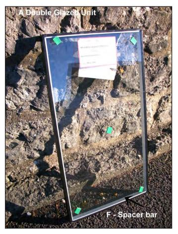
What actually happens is the perimeter edge of the unit loses its integrity and lets in moisture somewhere. Initially it may only be visible when the sun shines directly on it and heats the moisture within drawing it upwards and thus appearing as condensation. It will however, worsen over time until the unit is described as being totally broken down.
